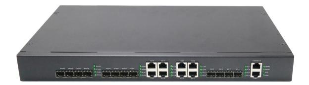
HA7308CX EPON OLT is a high integration and medium capacity cassette EPON OLT designed for operators' access and enterprise campus network. HA7308C provides 8 downlink 1.25G EPON ports, 8 \* GE LAN Ethernet ports and 4 \*10G SFP for uplink. The height is only 1U for easy installation and space saving. It adopts the advanced technology, offering efficient EPON solution. Moreover, it saves a lot cost for operators for it can support different ONU hybrid networking.
